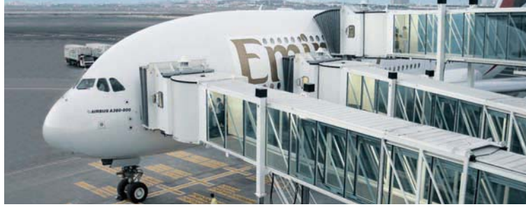
Boarding time of only 34 minutes – made possible by our passenger boarding bridges, developed specially for the Airbus A380 with “Apron Drive” to reach the upper deck.
